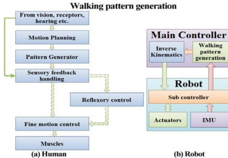
Figure 6: Block diagram of walking pattern generation in (a)human, (b)robot (D. et al., 2012)
