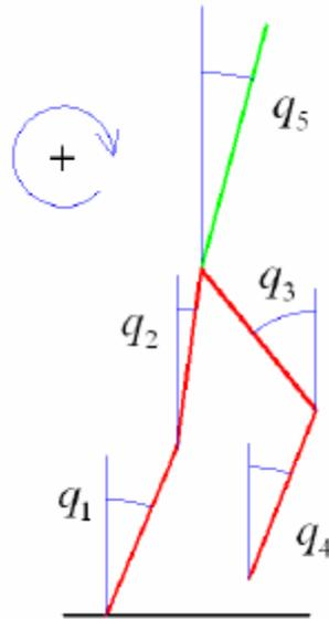
Figure 4: Configuration of a five-link bipedal walking robot(Zonfrilli, Oriolo, & Nardi, 2002)
