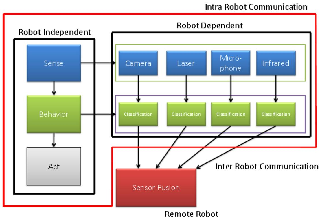
*Figure 8: Overview of communication structure*
