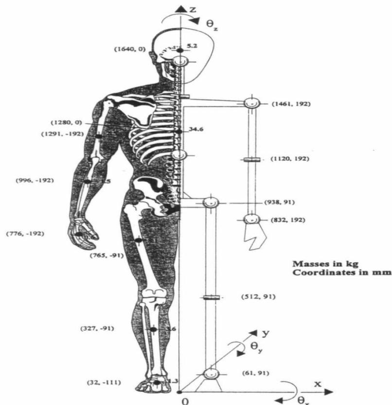
*Figure 1: Mass and centre of gravity of limbs (Right side) and principle joint coordinates (left side) (Seward et al., 1996)*
