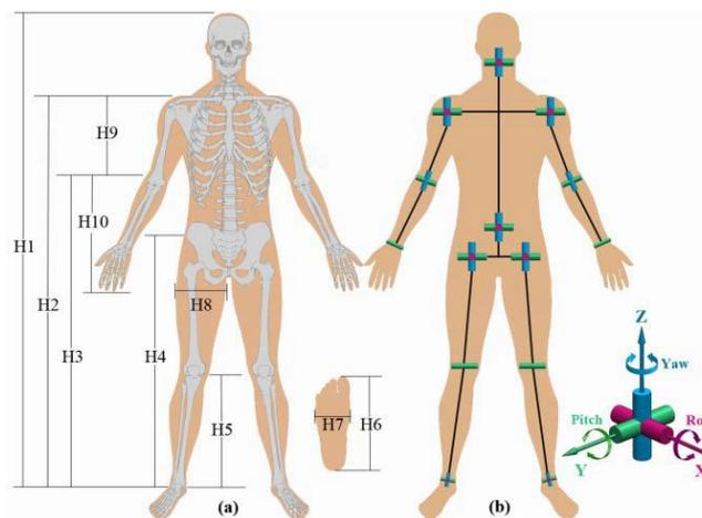
Figure 5: (a) Human dimensions, (b) kinematics diagram representing the DOF in human proportions (D., P., & M., 2012)
