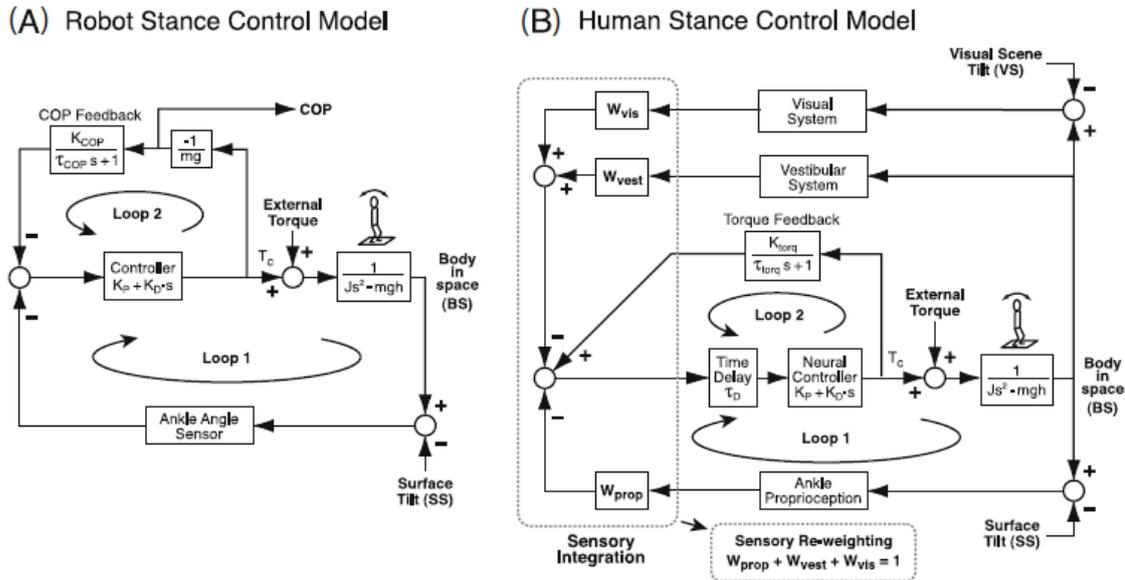
Figure 7: Block diagram model of robot stance control using ZMP compensation and a simplified model of human stance control(Peterka, 2009),
