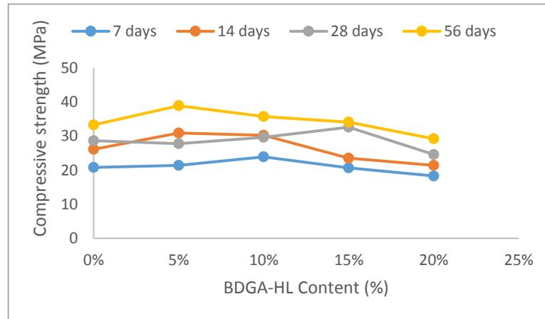
Figure 9 Compressive strength of BDGA-HL concrete at the curing days
