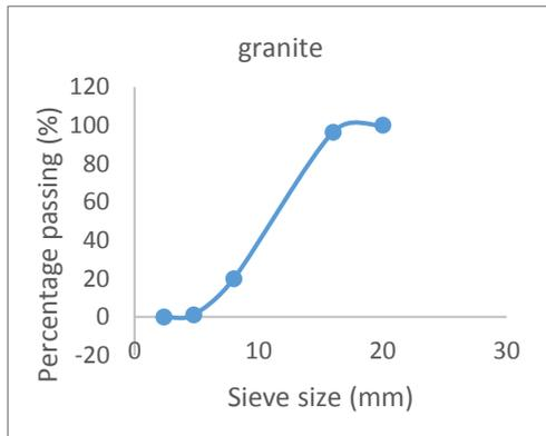
Figure 4 Particle size distribution of Coarse aggregate
