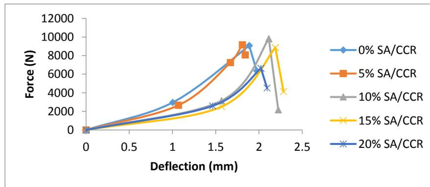
Figure 11 Flexural load, deflection curve of concrete beam specimens
