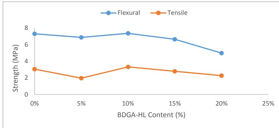
Figure 10 Flexural and split tensile strength of BDGA-HL concrete at 28<sup>th</sup> day curing
