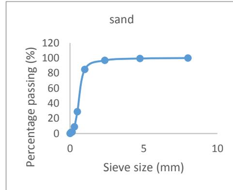
Figure 5 Particle size distribution of fine aggregate
