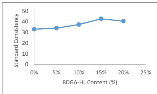
Figure 6 Standard consistency of BDGA-HL mortar
