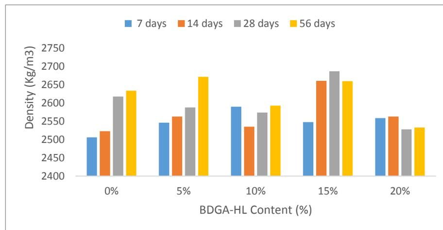
**Figure 8** Density of BDGA-HL concrete at the curing days
