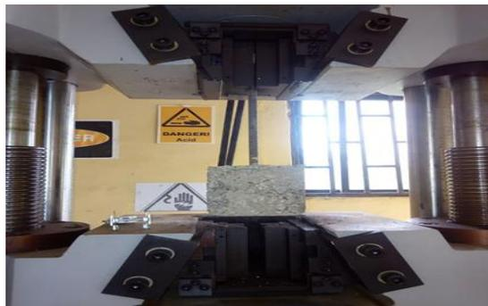
**Figure 1** Bond Stress Test Setup
