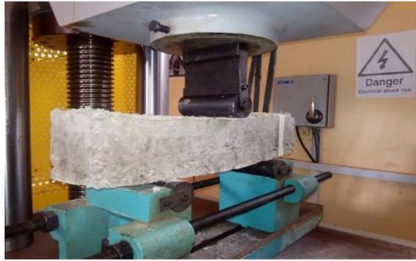
Figure 2 Specimen beam under flexural test
