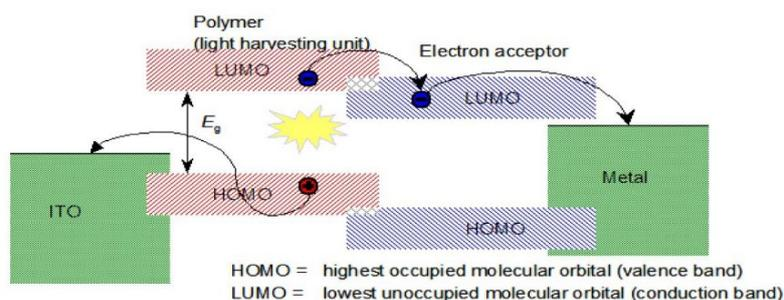
**Figure 3.** The working process in organic solar cell (Bagher, 2014a)
