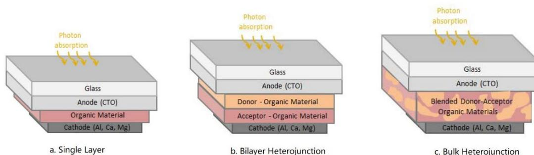
**Figure 2.** The basic structures of OPV solar cell for three types (Khalil et al., 2016)
